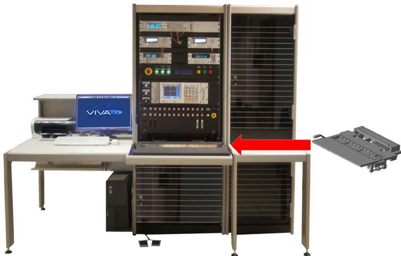
Figure 3: The first proposal from ATE suppliers is usually to build a fixture adaptor to be inserted between the new ATE receiver and the existing test fixtures.
