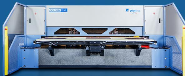
48" x 110" platform insures precision drilling/ routing over entire work area
