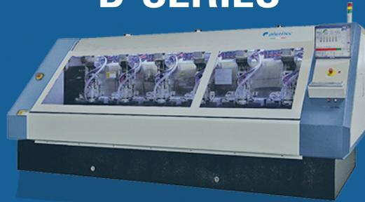
“D” Series 6-spindle driller/router is a proven, affordable workhorse
