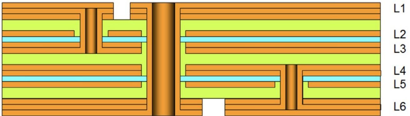
Figure 3: This 6-layer PCB stackup can use an ECM between L2 and L3, or between L4 and L5, to form a large embedded capacitor. A similar strategy could be used with packaging.
