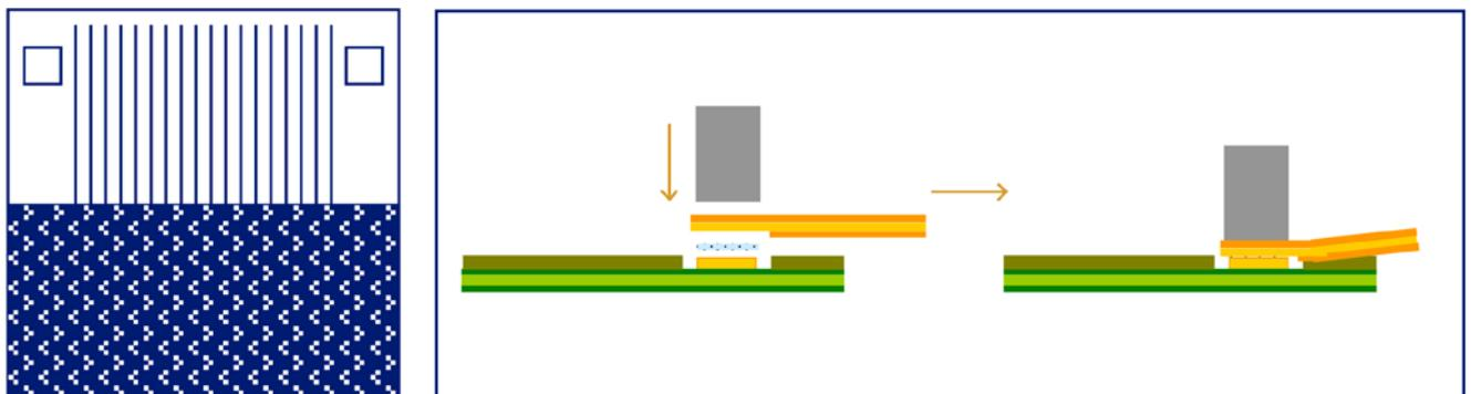
Figure 9: A preferred design with coverlay and resist removed from space around leads and bonding area.
