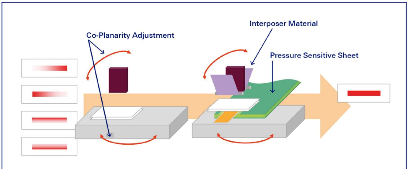
Figure 1: Prescale pressure measurement film can help operators address bonding imbalance issues.
