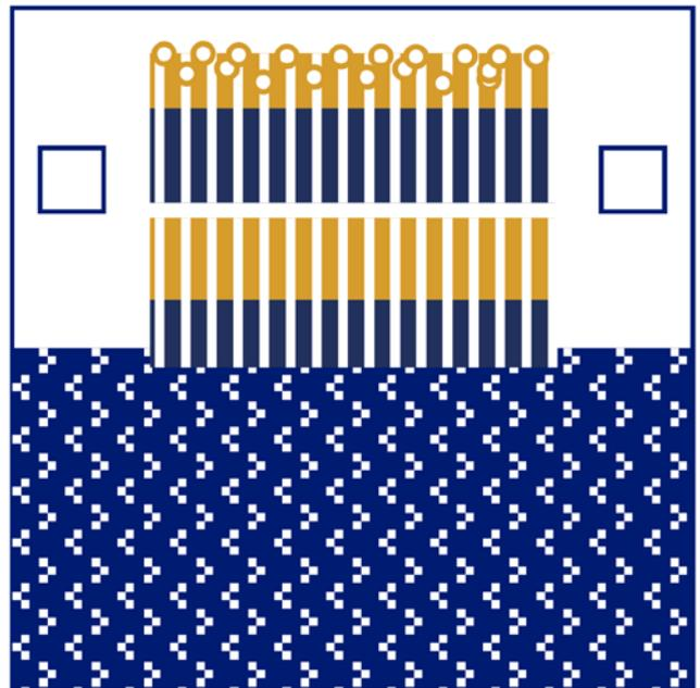
Figure 7: Example of the ACF bonding area on the center of two bonding lines, which can affect peel strength.
