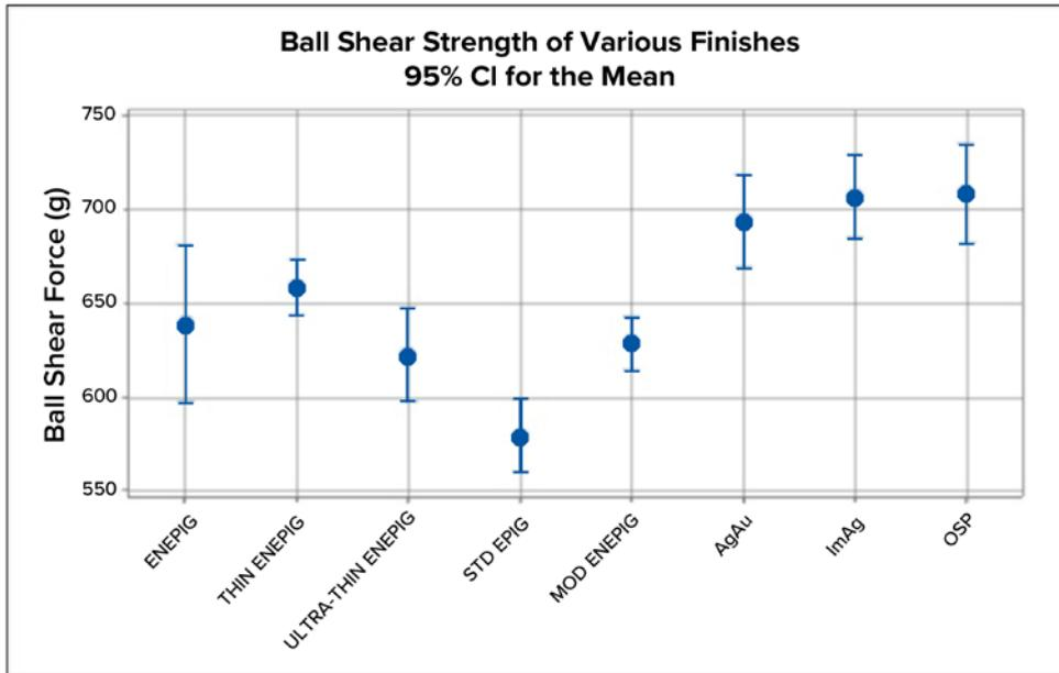
Figure 1: Interval plot of high-speed ball shear strength of various surface finishes.
