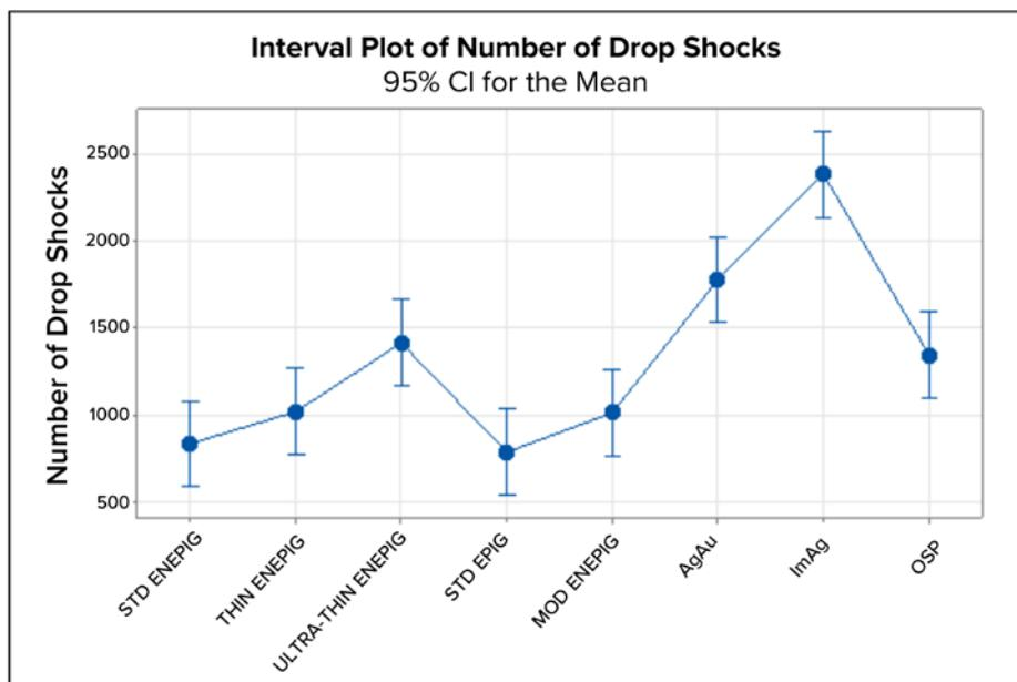
Figure 2: Interval plot of drop shock performance of various surface finishes.
