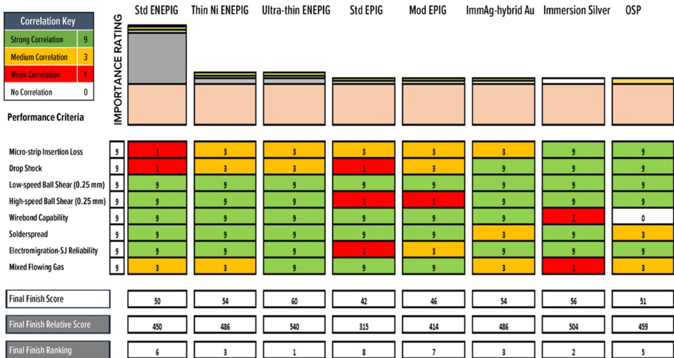
Figure 5: Quality function deployment (QFD) matrix of various surface finishes.
