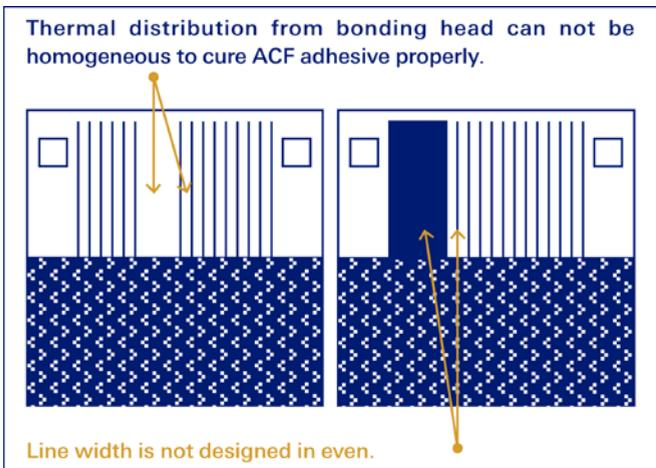
Figure 4: A poor design. Different thermal conductive lead widths will complicate temperature verification.
