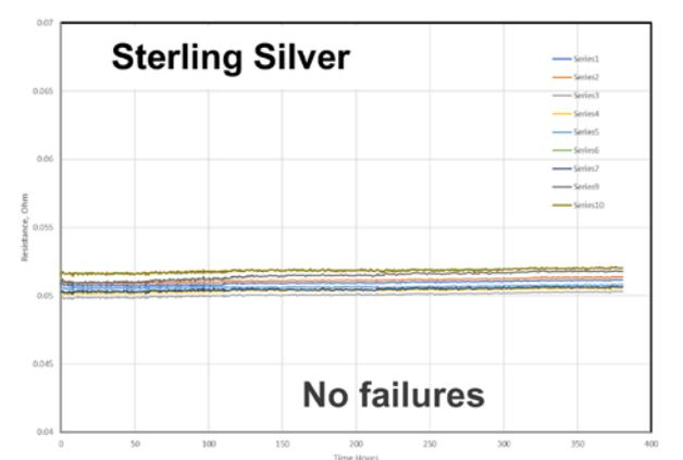
Figure 3: Resistance vs. time in electromigration test in the test vehicle plated with different surface finishes.
