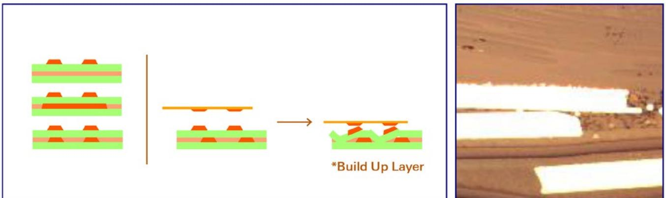
Figure 2: The preferred design (left), and not preferred (right). Alignment is critical.
