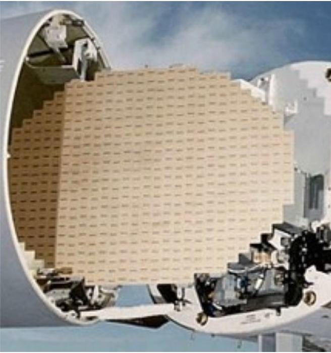
Figure 1: An example of a flat-panel active electronically steered array (AESA) radar system.
