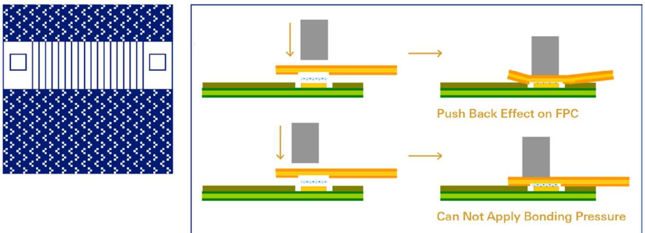
Figure 10: An example of a non-preferred design showing the results when coverlay and resist are not removed correctly.
