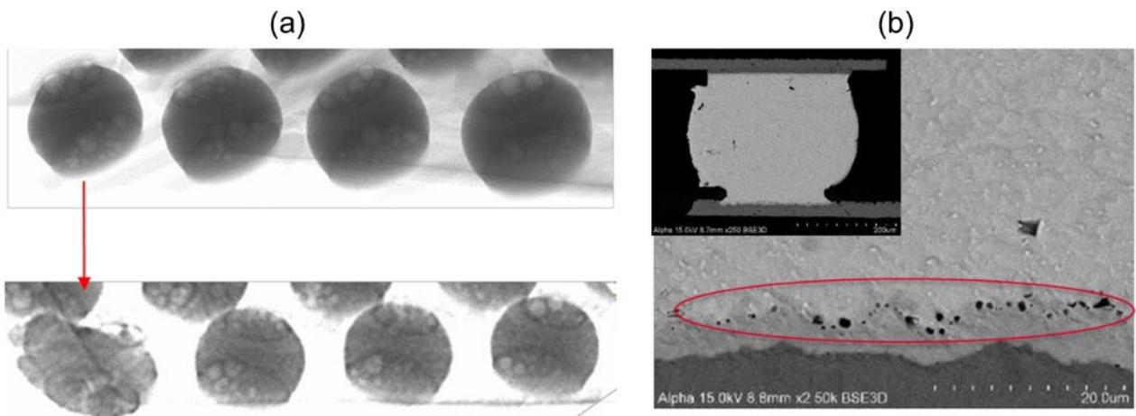
Figure 4: X-ray imaging of standard EPIG solder joints before and after electromigration test.
