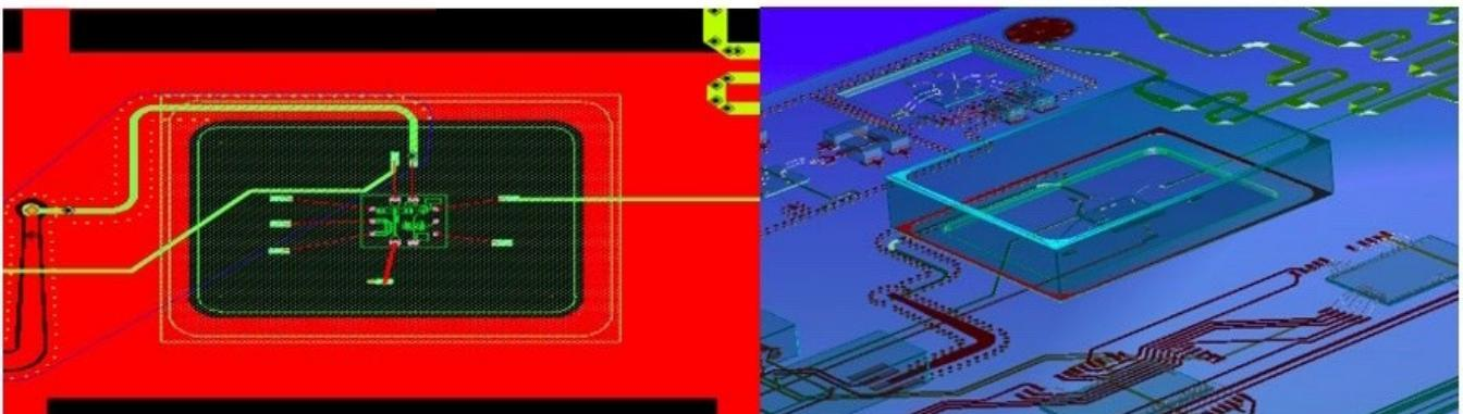
Figure 3: Example of intelligent cavity design object during layout.
