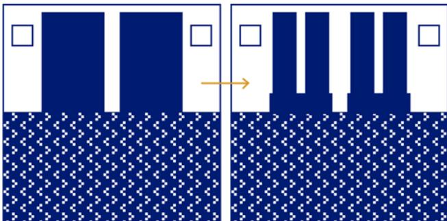
Figure 5: With large line widths, large gold areas are not necessary.
