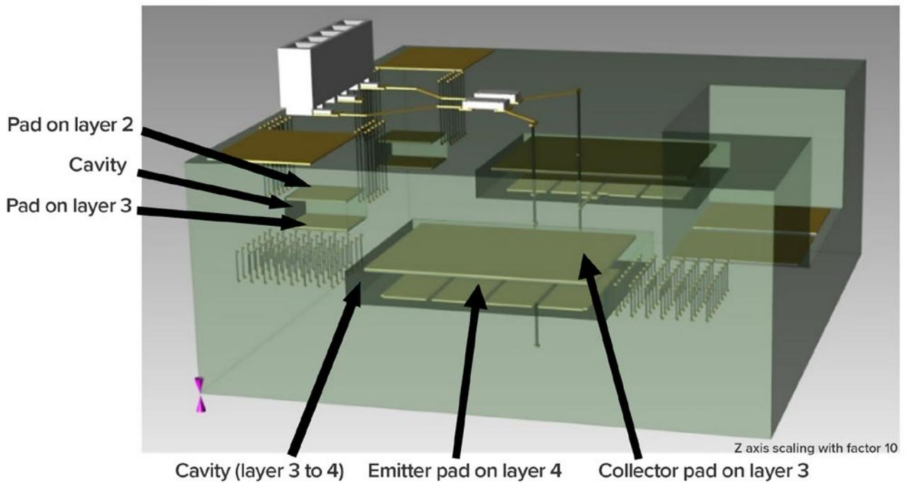
Figure 2: A 3D view of embedded components.
