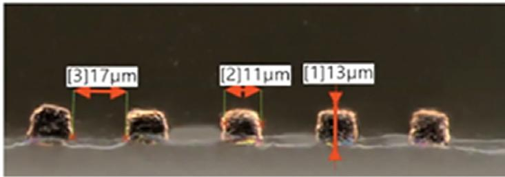
Substrate is 100 µm thick LCP, copper traces are 11 µm wide, 13 µm thick, with 17 µm spacing.
