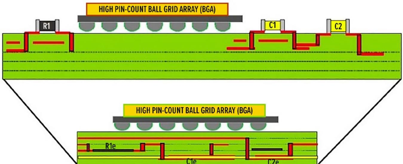
Figure 1: Embedded passive components reduce size and space.
