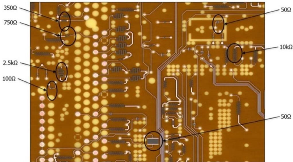
Figure 2: A PCB with varying resistor values of 100 ohms/square.
