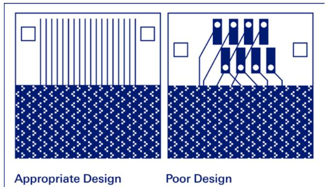
Figure 6: A good design (left) and a poor design (right). The poor design may cause partial compression, because only the crossing point could be compressed on the back side of the flex circuit.
