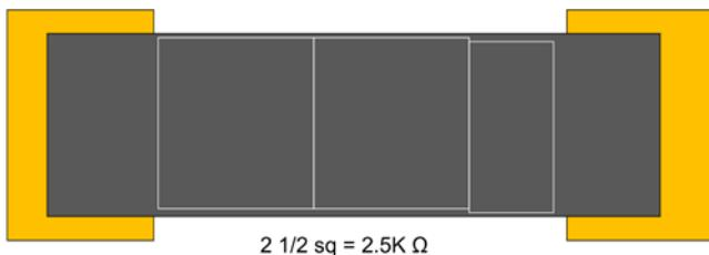
Figure 2: Basic “bar” thick-film resistor element design.
