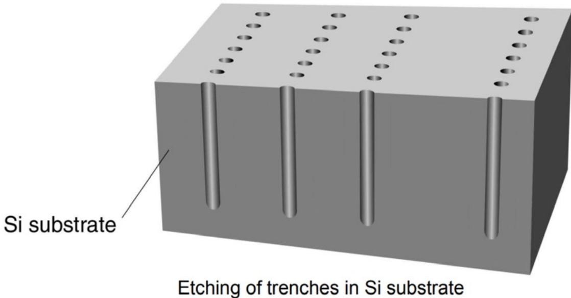
Figure 5: Silicon trench capacitors on Si substrate.
