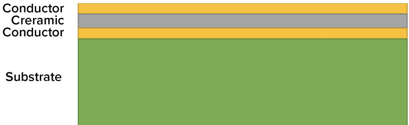
Figure 4: Embedded ceramic film structure for a package substrate/interposer.
