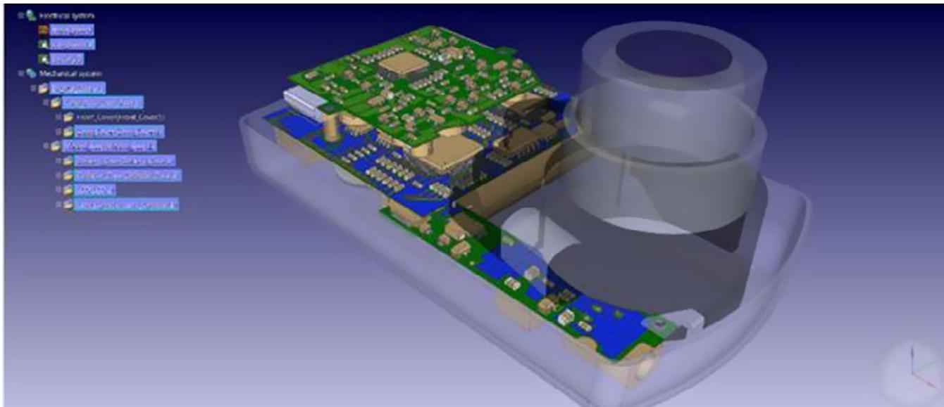
Figure 3: 3D multi-board design promotes electrical-mechanical collaboration.
