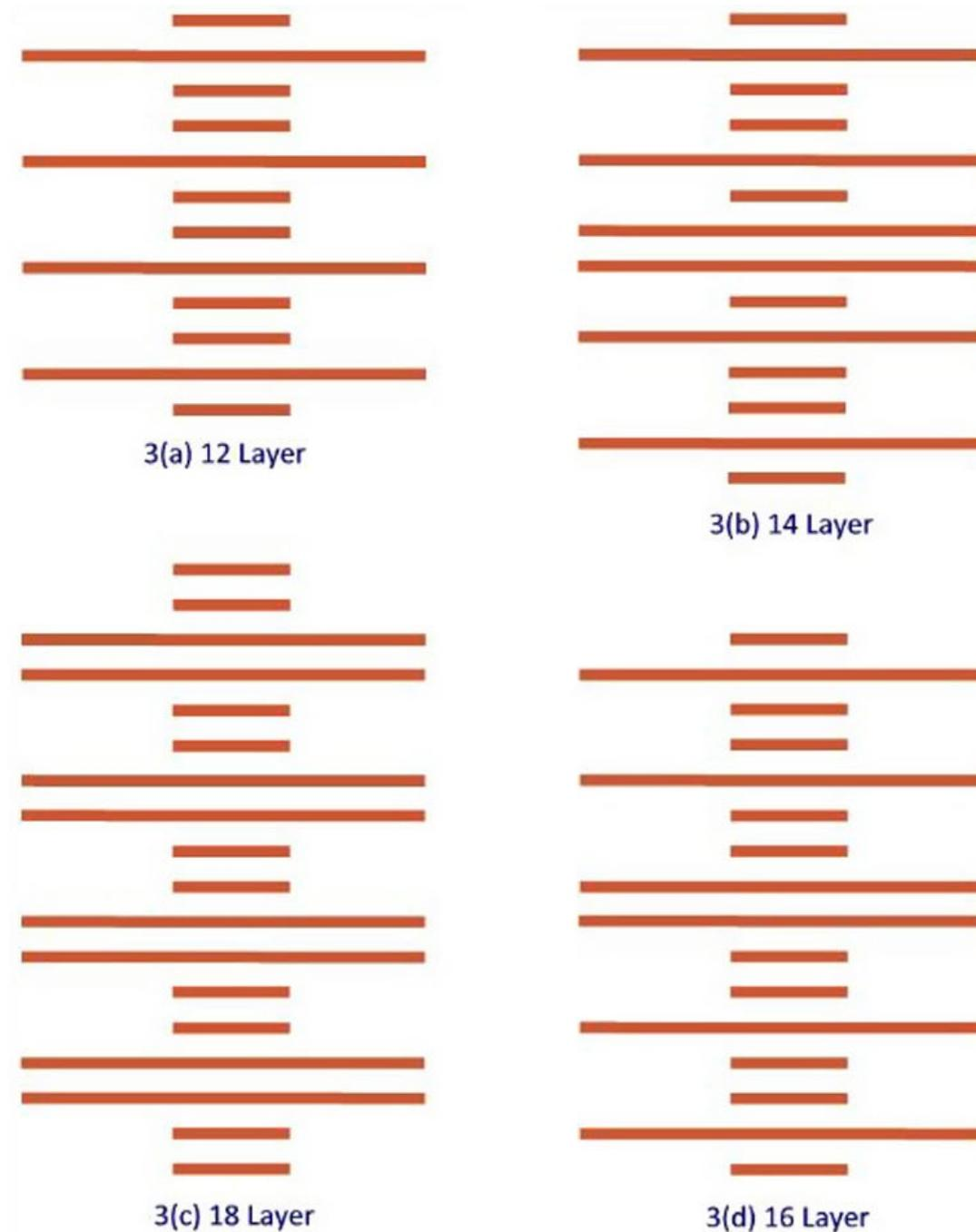
Figure 3: Image illustrating the signal/plane configuration for 12–18 layers.
