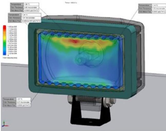
Figure 7: The thermal simulation also shows the movement of the condensation film caused by gravity.
