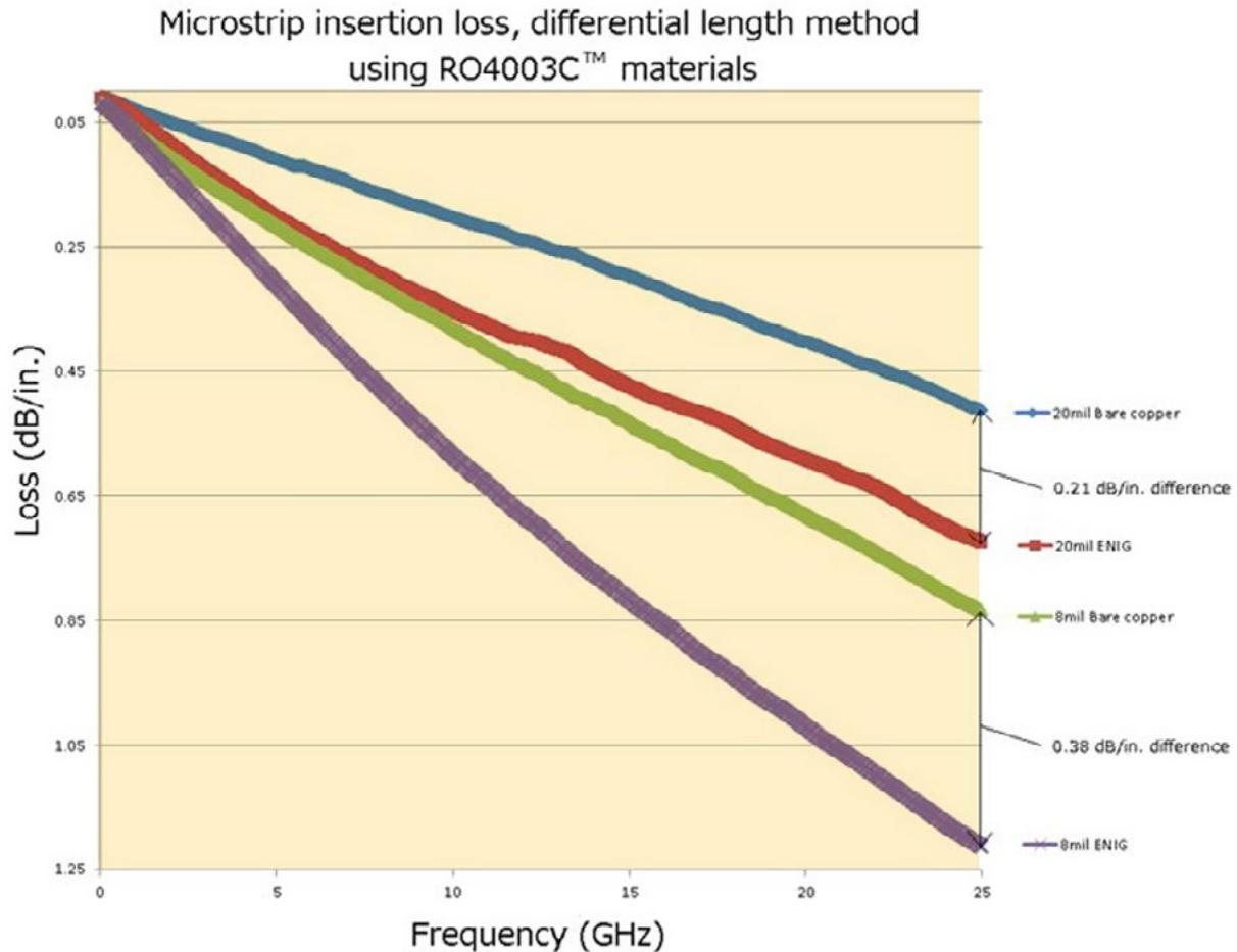
Figure 1: Results of experiment showing difference in insertion loss of microstrip transmission line circuit using bare copper and ENIG, with different substrate thickness.
