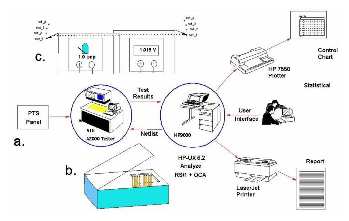
Figure 2: (a) HP's PTS arrangement with a continuity tester, (b) coupon test fixture for individual coupons, (c) milliohm measurement using a 1-amp power supply and digital panel meter in a Kelvin four-wire test configuration.
