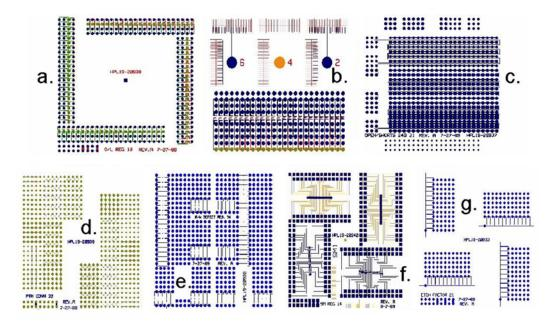
Figure 1: The seven coupons designed by HP; (a) Outer layer registration in 0.00025" increments, (b) inner layer registration and shifting in 0.00025" increments, including 0.1-mil X-ray vernier, (c) trace/trace/pad open and short circuit on multiple layers, (d) PTH continuity patterns, including I/L connections at various angles to the PTH, (e) artwork defects analysis in 0.00025" increments, and (f) etch factor analysis in 0.00025" increments.
