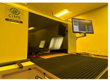
ICM runs each board through an AOI system, resulting in higher first-pass yields.
