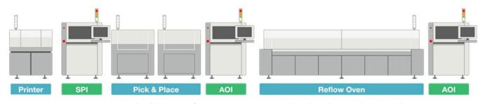
Figure 1: An example of a line configuration to improve yield with multipoint data correlation.
