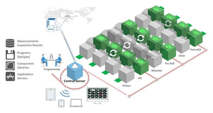
Figure 4: Factory connectivity example using KSMART.
