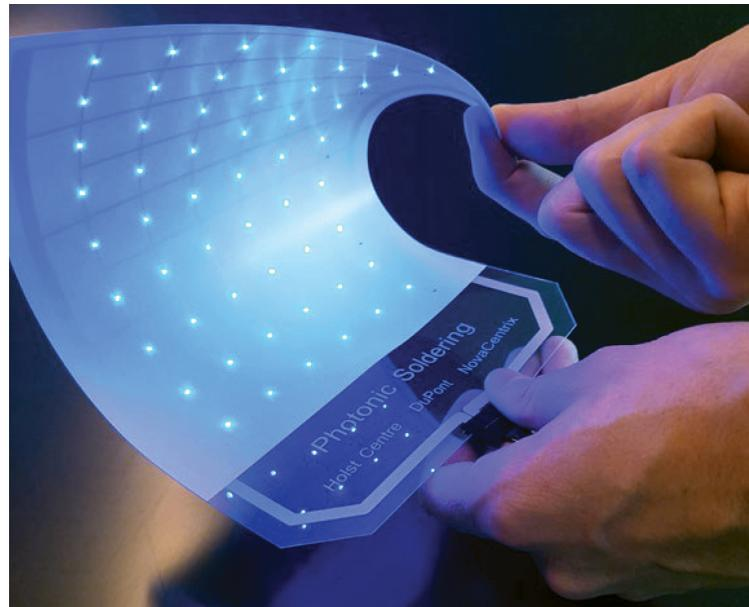
Photonic soldering allows standard lead-free solder to be cured on low-melting-point plastic films in a matter of seconds.
