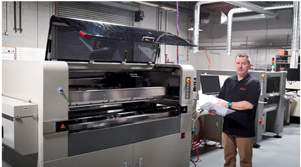
Figure 2: Online training on SMT fully automatic stencil printer.
