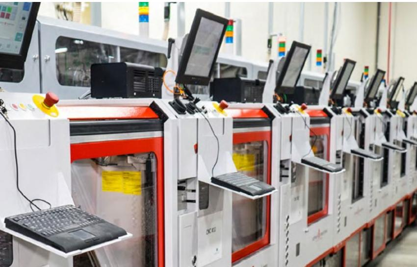
Schmolz single-spindle drilling machines in tandem.
