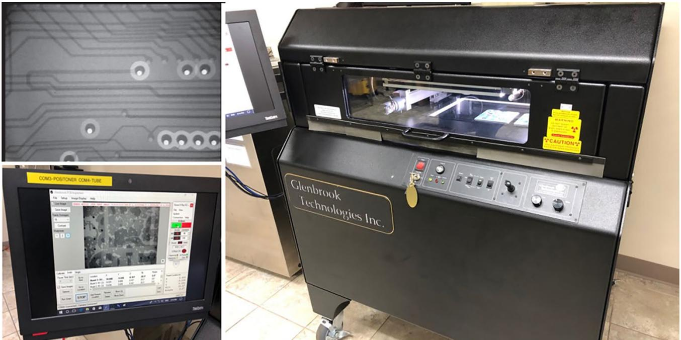
the Ram Optical Sprint MVP 600 stands for 600 mm, or 23.6” in the X-axis, so full panel inspection is now a reality. The full specifications for the size are X-axis 600 mm (23.6”), Y-axis (17.7”), and Z-axis (5.9”), which is quite impressive and can handle most any measurement a shop would need.
