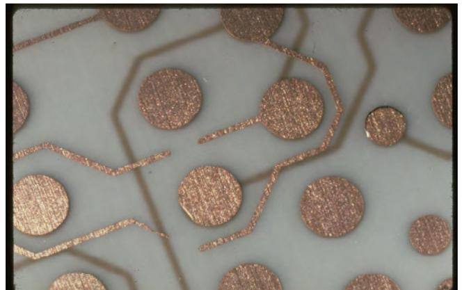
Figure 1: Short circuit (left) and open circuit (right) due to insufficient resist adhesion.
